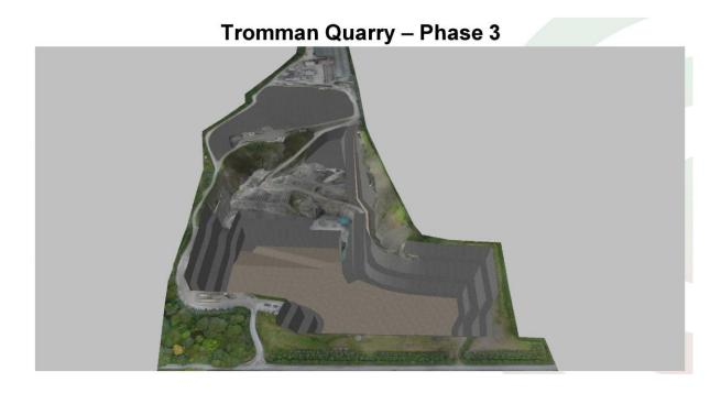
Simultaneously to the removal of the overburden into its final resting place in the floor the 3 upper benches will be developed in a northerly direction, to achieve the maximum extents of the designed footprint of the quarry, as illustrated overleaf. Tromman Quarry - Phase 3
